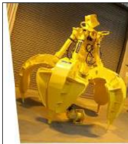
Figure 15: Example grab attached at the end of the crane.
